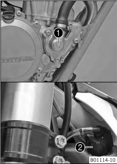
Water pump ❶ in the engine circulates the coolant. The pressure resulting from the warming of the cooling system is regulated by a valve in radiator cap ❷. This ensures that operating the vehicle at the specified coolant temperature will not result in a risk of malfunctions.
