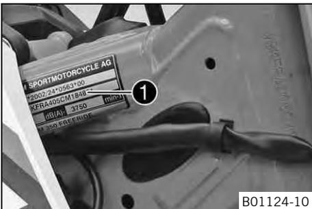
The type label ❶ is fixed to the frame at the front right.
