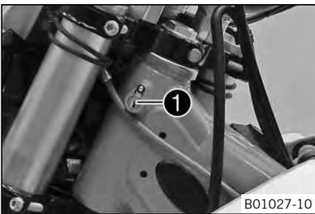
Steering lock ❶ is fitted on the left side of the steering head. The steering lock is used to lock the steering. Steering, and therefore riding, is no longer possible.
