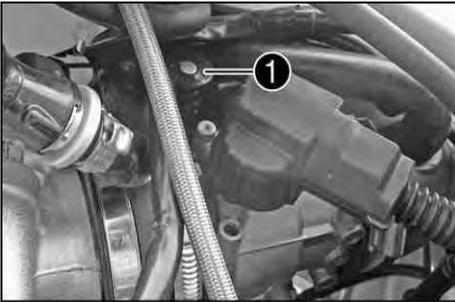
Idle speed adjusting screw ❶ is located on the throttle valve body at the top left. The idle speed adjusting screw has two functions. Turning it controls the idle speed. Pulling it out all the way raises the idle speed during a cold start.
