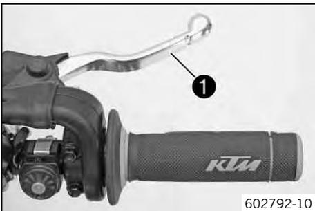
Hand brake lever ❶ is located on the right side of the handlebar. The front brake is engaged using the hand brake lever.
