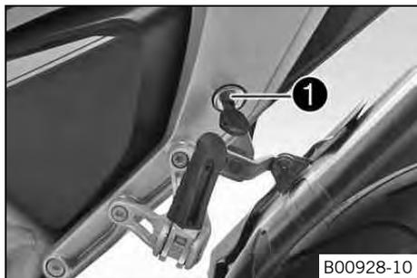
The seat lock **1** is located on the left side of the vehicle. It can be locked with the ignition key.
