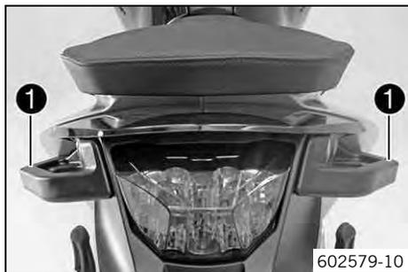
The handrails ① are used for moving the motorcycle around.
