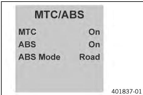
The traction control lowers the tightening torque in case of loss of traction in the rear wheel. Depending on the traction control setting, a slight slip on the rear wheel may be desirable. Example: Offroad.
