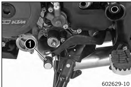
The shift lever ❶ is fitted on the left side of the engine.
