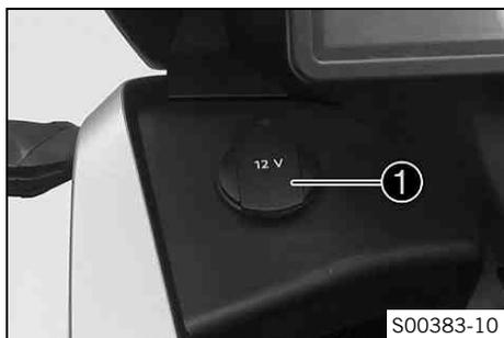
Socket ❶ for electrical accessories is fitted to the left of the combination instrument. It is connected to permanent positive and fuse-protected.
