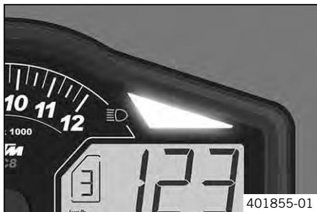
The shift warning light flashes or lights up when the transmission should be shifted. In the **"Shift Light"** menu, the engine speed for the shift warning light can be set. The shift warning light flashes over **"RPM1"** and lights up permanently over **"RPM2"**.
