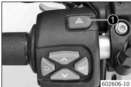
The hazard warning flasher switch ① is fitted on the combination switch on the left. The hazard warning flasher is used to indicate emergency situations.
