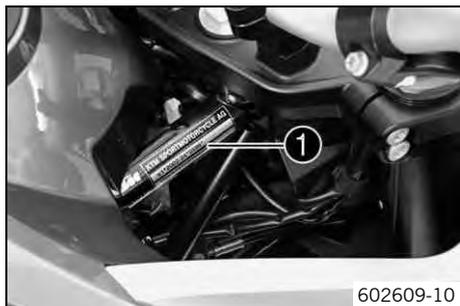
The type label **1** is on the top right of the frame behind the steering head.
