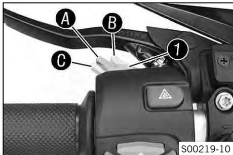
The light switch ① is fitted on the combination switch on the left.
