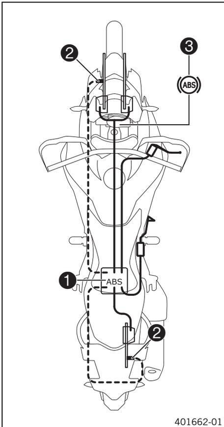
The ABS unit **1**, which consists of a hydraulic unit, ABS control unit, and return pump, is installed under the seat. A wheel speed sensor **2** is located at the front and rear wheels.
