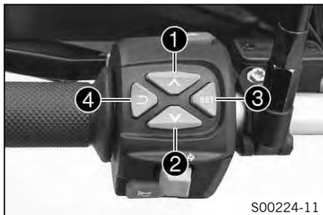
The menu switch is fitted in the middle of the left combination switch. The menu buttons are used to control the matrix display on the combination instrument.
