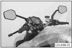
Mount and tighten the rear mirror on both sides.
