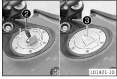
Press down the filler cap and turn back ignition key 2 until the fuel tank lock locks.
