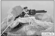
Remove the controls from the transport holder. Remove the screws of the handlebar clamp. Take off the handlebar clamp and transport holder.
