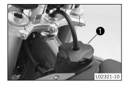
Turn filler cap 1 counterclockwise and lift it off.
