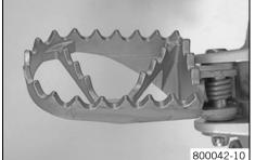
Mount the footrests with the springs and pins. Secure the pins using the washers and cotter pins.
