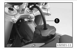
Mount filler cap and turn it clockwise until the fuel tank is tightly closed.
