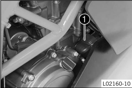
Water pump ① in the engine circulates the coolant.
