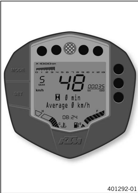
The temperature display consists of 13 bars. The more bars that light up, the hotter the coolant. When all bars light up, the following warning note appears on the info display:
