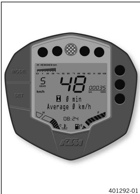
The filling level display consists of 9 bars. The more bars are lit, the more fuel is in the fuel tank.
