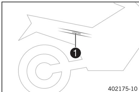
The chassis number **1** is stamped on the right side of the frame under the seat.
