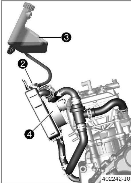
The coolant is cooled by the air stream and a radiator fan ④, which is controlled by a thermostat.
