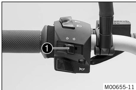
The turn signal switch **1** is fitted on the left side of the handlebar.
