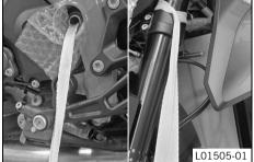
Carefully loosen and remove the tensioning belt from the frame.
