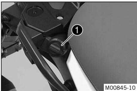
The passenger seat heating switch **1** is located next to the right grab handle.
