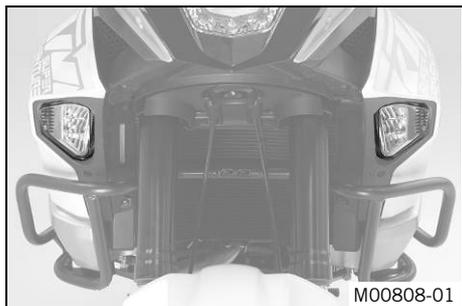
The cornering headlight is located to the left and the right in the side cover.
