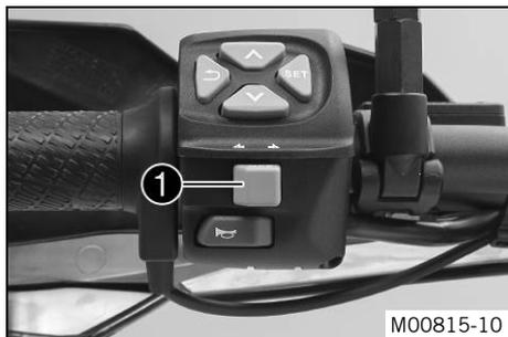
The turn signal switch ① is fitted on the combination switch on the left.
