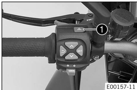
The hazard warning flasher switch **1** is fitted on the combination switch on the left. The hazard warning flasher is used to indicate emergency situations.
