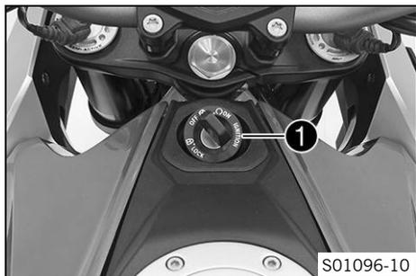
The ignition/steering lock ❶ is located in front of the upper triple clamp.
