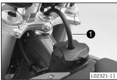
Mount filler cap and turn it clockwise until the fuel tank is tightly closed.
