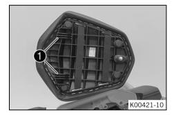
Hook catches **(1)** of the passenger seat onto the storage compartment, lower the rear, and simultaneously push forward.
