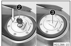
Press down the filler cap and turn back ignition key 2 until the fuel tank lock locks.
