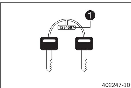
The key number ① for the steering lock is stamped onto the key connector.
