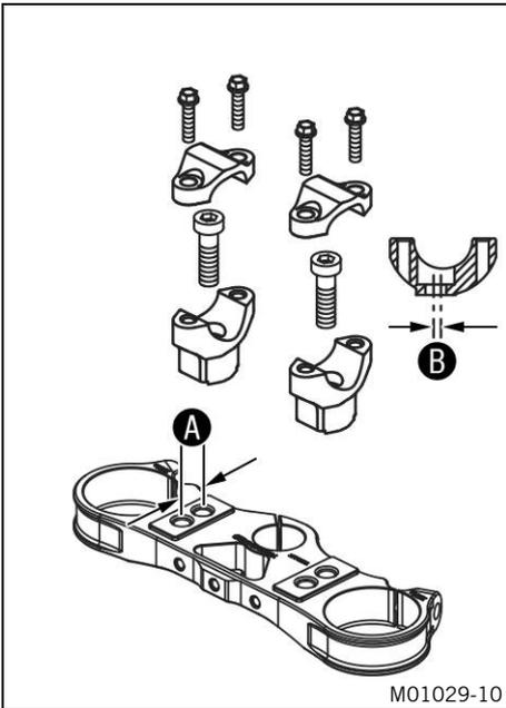
On the upper triple clamp, there are two holes at a distance of **A** to each other.
