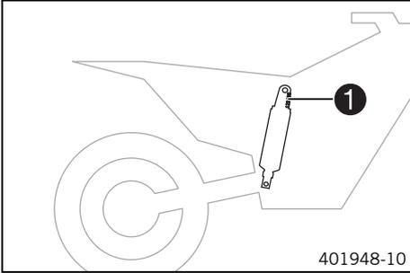
The shock absorber part number ① is stamped on the top of the shock absorber above the adjusting ring towards the engine side.
