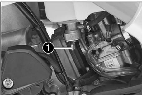
The fuel tap is attached to the left side of the fuel tank.
