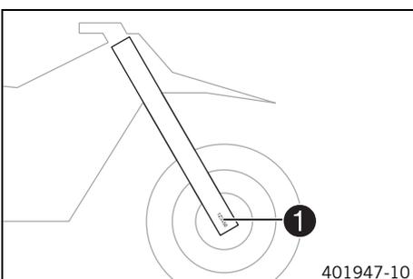
The fork part number ① is stamped on the inner side of the axle clamp.
