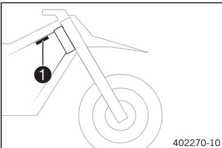
The type label ① is mounted on the frame at the front right.
