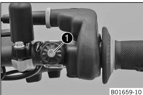
Electric starter button ① is fitted on the right side of the handlebar.
