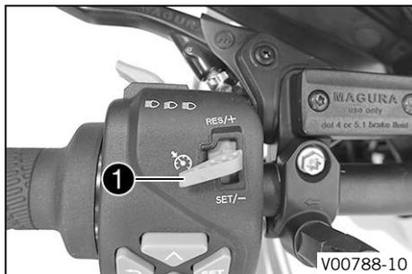
The cruise control system tip switch ① is fitted on the left side of the combination switch.
