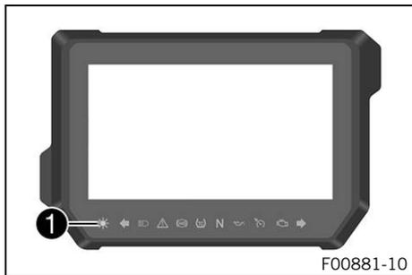
The electronic immobilizer secures the vehicle against unauthorized use. The immobilizer is activated and the engine electronics are locked as soon as the ignition is switched off via the Race-on button (🔑 p. 34).
