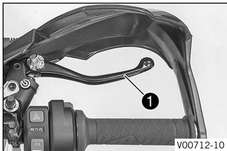
The hand brake lever ❶ is fitted on the right side of the handlebar. The hand brake lever is used to activate both the front brake and rear brake at the same time.
