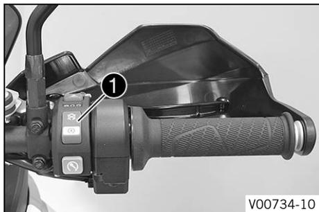
The emergency OFF switch/electric starter button ❶ is fitted on the right side of the combination switch.
