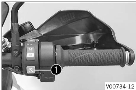
The Race-on button ① is fitted on the right side of the combination switch.
