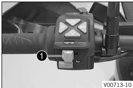
Turn signal switch ❶ is fitted on the combination switch on the left.
