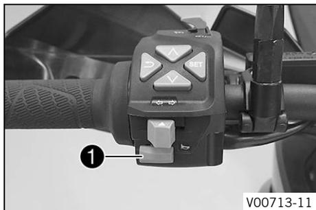
The horn button ① is fitted on the combination switch on the left.
