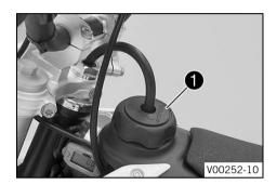
Turn the tank cap 1 counterclockwise and pull it up.
