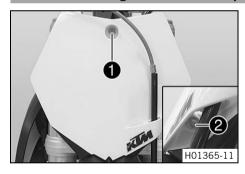
Position the start number plate. Mount and tighten screw ①. Guideline
