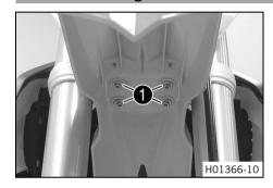
Position the front fender. Mount and tighten screws ①.
