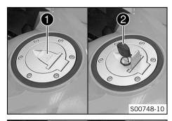
Lift cover 1 of the filler cap and insert ignition key 2 in the fuel tank lock.
