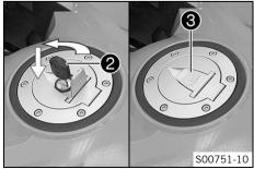
Push down the filler cap and turn the ignition key counterclockwise until the tank lock closes.
