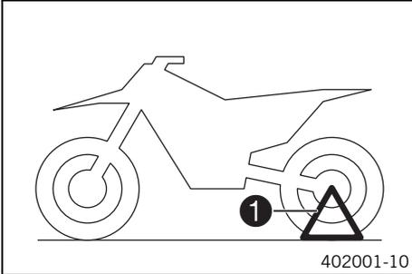
The holder for plug-in stand ❶ is on the left side of the wheel spindle. The plug-in stand is used to park the motorcycle.
