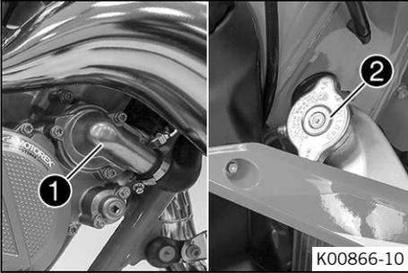
Water pump **1** in the engine ensures forced circulation of the coolant. The pressure resulting from the warming of the cooling system is regulated by a valve in radiator cap **2**. This ensures that operating the vehicle at the specified coolant temperature will not result in a risk of malfunctions.
