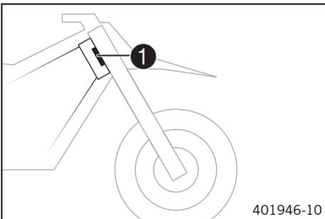
The type label ① is fixed to the front of the steering head.
