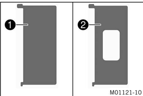
The radiator cover is installed in front of the left radiator, depending on the ambient temperature.
