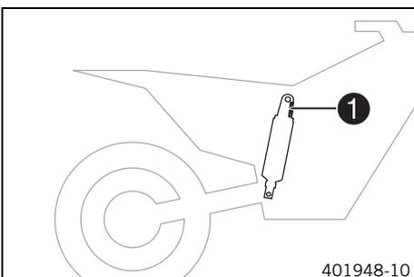
Shock absorber article number ① is stamped on the top of the shock absorber above the adjusting ring towards the engine side.
