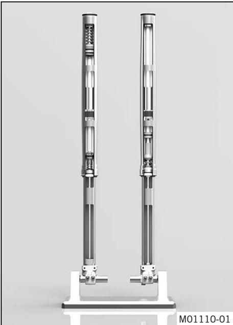
Air suspension **WP Performance Systems AER 48** is used in the fork. In this system, suspension is located in the left fork leg and damping in the right fork leg. As fork springs are no longer required, a significant weight advantage is achieved when compared to conventional forks. The response on slightly uneven surfaces is significantly improved. In normal driving mode, suspension is provided exclusively by an air cushion. A steel spring is located in the left fork leg as an end stop.
