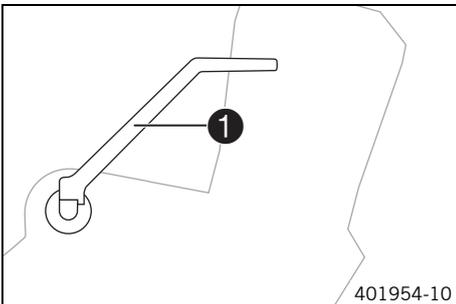
Kick starter **1** is fitted on the right side of the engine. The top part of the kick starter pivots.
