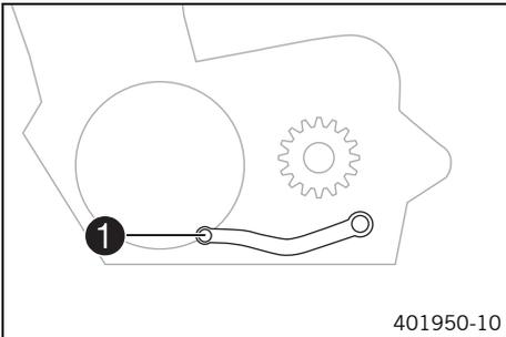
Shift lever **1** is mounted on the left of the engine.
