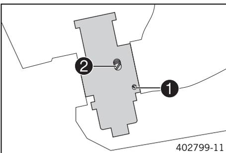
– Screw in idle air adjusting screw **1** all the way and turn it to the specified basic position.
