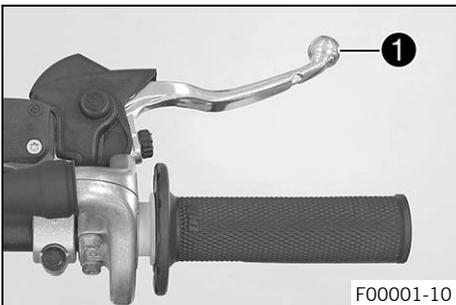
Hand brake lever ❶ is fitted on the right side of the handlebar.
