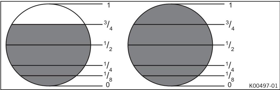
When the throttle slide is 3/4 open, the influence of the main jet is greatest. The clip position and the idling jet have only minimal influence.
