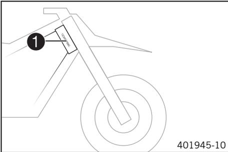
The chassis number ① is stamped on the right side of the steering head.
