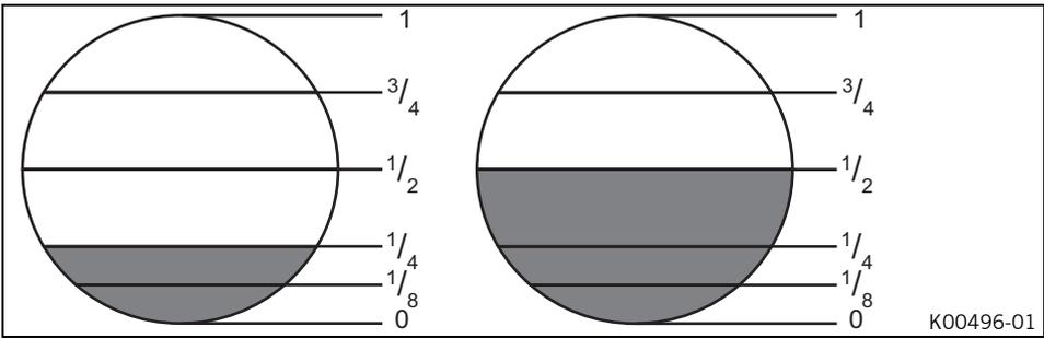
When the throttle slide is 1/4 open, the idling jet and the clip position have the greatest influence. The influence of the first cylindrical part of the needle is less.
