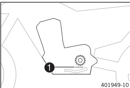
The engine number ① is stamped on the left side of the engine under the engine sprocket.
