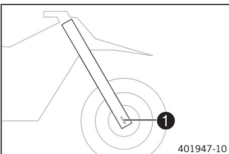
The fork part number ① is stamped on the inside of the axle clamp.
