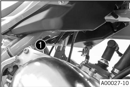
Plug-in connector **1** of the ignition timing map adjustment is located on the frame under the fuel tank.
