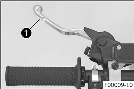
Clutch lever ❶ is fitted on the handlebar on the left.
