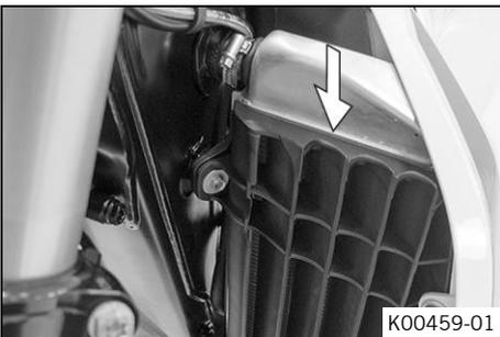
The radiator cover is mounted in front of the left radiator between the radiator shield and radiator.
