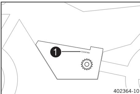
The motor number ❶ is located on the left side of the motor over the motor sprocket.
