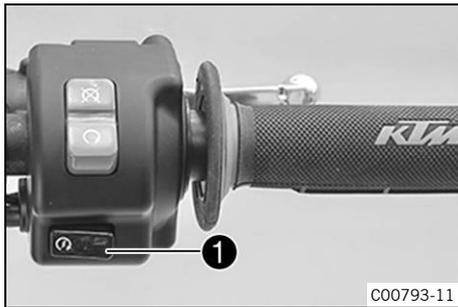
The start button **1** is fitted on the right side of the handlebar. The start button is only enabled when the main switch is switched on.
