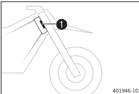
The type label ❶ is located on the front steering head.
