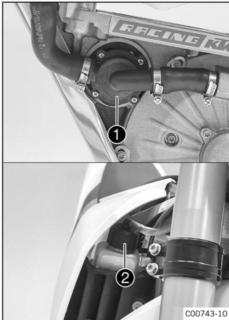
When the vehicle is in standby mode, the water pump **1** pumps the coolant through the cooling circuit. The pressure in the cooling system increases with the temperature of the coolant. A safety valve is contained in radiator cap **2**. This ensures that operating the vehicle at the specified coolant temperature will not result in a risk of malfunctions.
