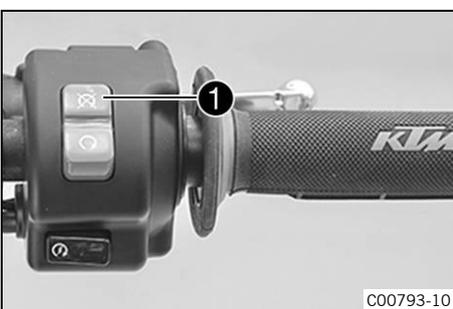
The main switch **1** is attached to the right side of the handlebar. The main switch is also used as an emergency OFF switch.
