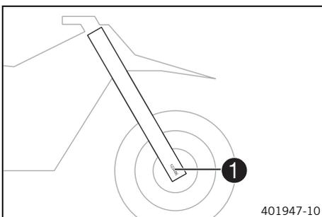
The fork part number ❶ is stamped on the inner side of the axle clamp.
