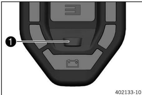
The map-select tip switch ❶ determines the driving mode.
