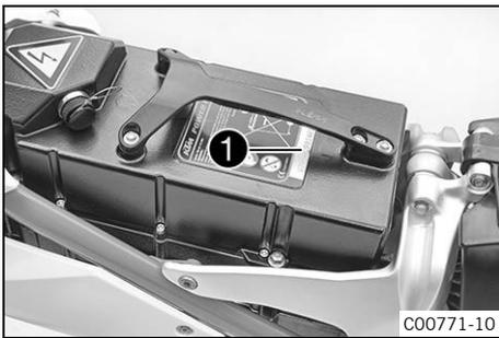
The battery identification number (**BIN**) **1** is stamped under the handle of the KTM PowerPack.
