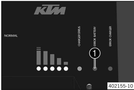
The faults are indicated by LED ❶ on the battery charger. All of the following blink codes are displayed on the charger and refer to the KTM PowerPack.
