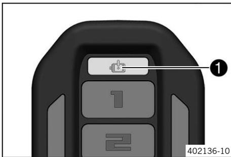
The faults are indicated by the yellow electric motor indicator lamp ❶ and by acoustic signals that sound at the same time.
