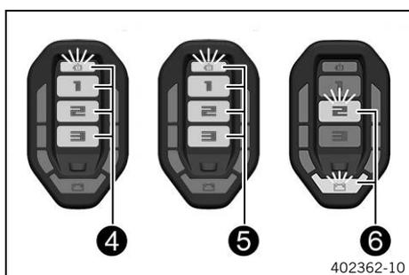
**All three driving mode indicators light up and the yellow electric motor indicator lamp (MIL) 4 flashes (blink code 22, 23, or 24):**
