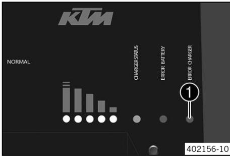
The faults are indicated by LED ① on the battery charger. All of the following blink codes are displayed on the charger and refer to the charger itself.
