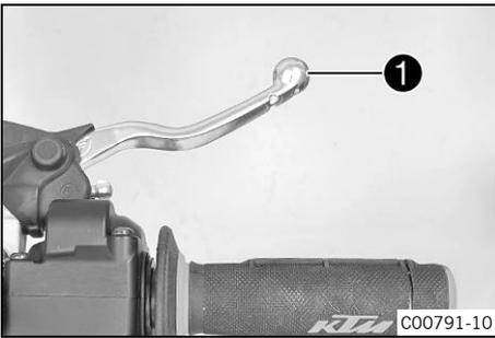
The front brake handle **1** is fitted on the right side of the handlebar.
