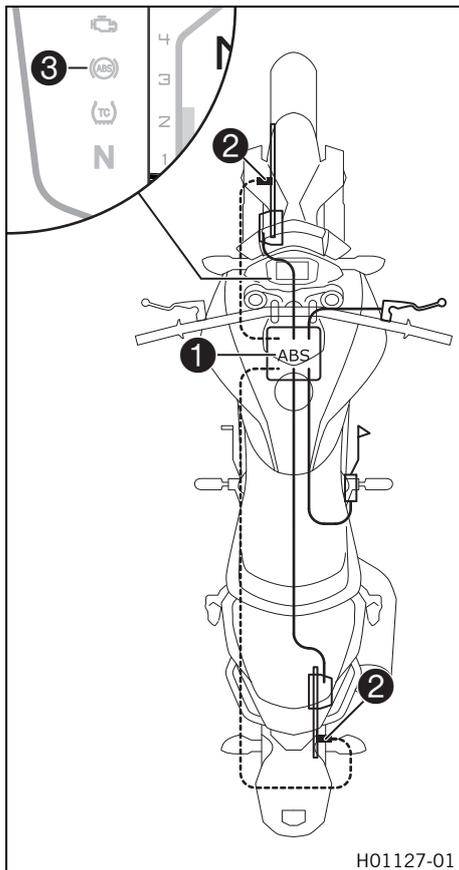
ABS unit **1**, which consists of a hydraulic unit, ABS control unit, and return pump, is installed under the fuel tank. One wheel speed sensor **2** is located in each case on the front and the rear wheel.
