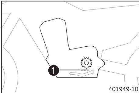
The engine number **1** is located on the left side of the engine under the engine sprocket.
