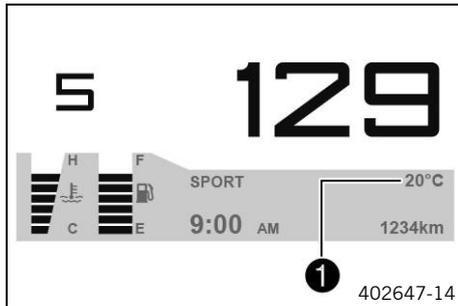
The current ambient temperature is shown in area ❶ of the display.
