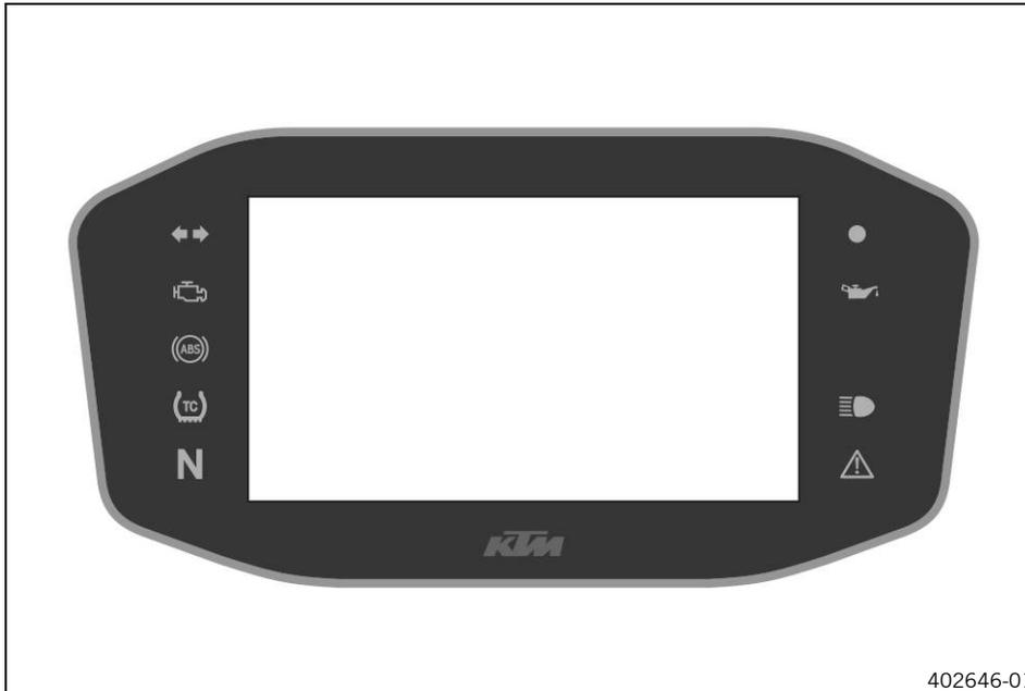
The indicator lamps offer additional information about the operating state of the motorcycle. When the ignition is switched on, all indicator lamps light up briefly.
