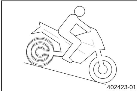
The **MSR** is an optional auxiliary function of the engine control. If the engine braking effect is too great, the **MSR** prevents the rear wheel from locking.
