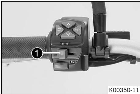
The turn signal switch ① is fitted on the left side of the handlebar.
