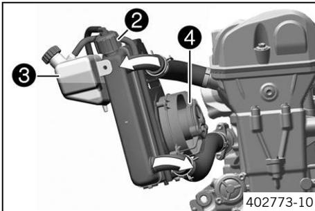
The coolant is cooled by the air stream and a radiator fan ❹, which is controlled by a thermostich.
