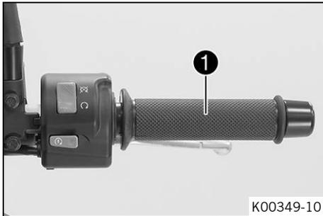
The throttle grip **1** is fitted on the right side of the handlebar.
