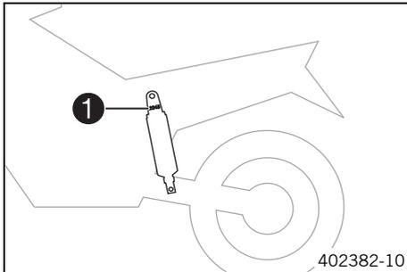
Shock absorber article number **1** is on the left side of the shock absorber.
