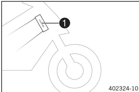
The chassis number **1** is stamped on the right side of the steering head.
