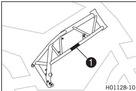
The type label USA **1** is located on the right side of the frame.
