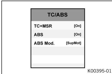
The traction control (TC
