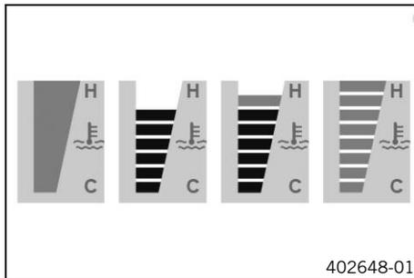
The temperature display consists of 8 bars. The more bars that light up, the hotter the coolant.
