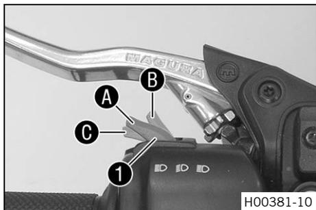
Light switch ❶ is fitted on the left side of the handlebar.
