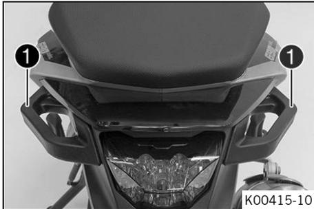
The handrails **1** are used for moving the motorcycle around. When you have a passenger, the passenger can hold on to the handrails during the journey.
