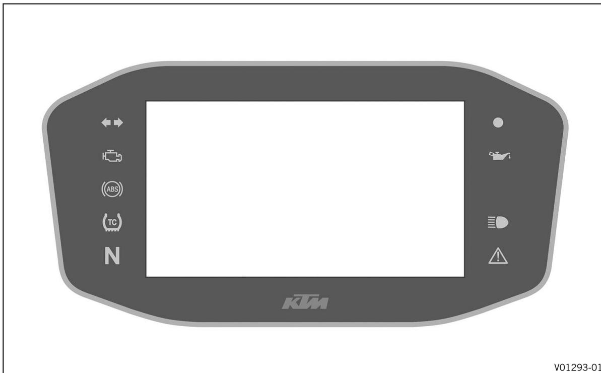
The indicator lamps offer additional information about the operating state of the motorcycle. When the ignition is switched on, all indicator lamps light up briefly.
