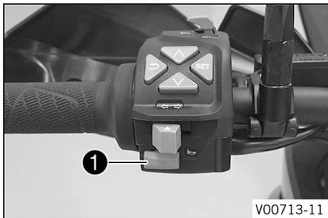
The horn button ❶ is fitted on the combination switch on the left.
