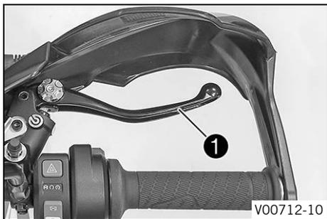
The hand brake lever **1** is fitted on the right side of the handlebar. The hand brake lever is used to activate both the front brake and rear brake at the same time.
