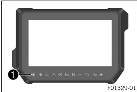
The Race-on indicator lamp **1** can indicate errors by flashing. The flashing occurs for up to five seconds after actuating the Race-on tip switch.
