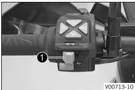
Turn signal switch **1** is fitted on the combination switch on the left.
