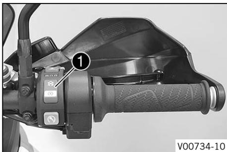
The emergency OFF switch/electric starter button **1** is fitted on the right side of the combination switch.
