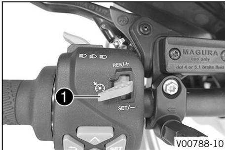
The cruise control system tip switch ❶ is fitted on the left side of the combination switch.
