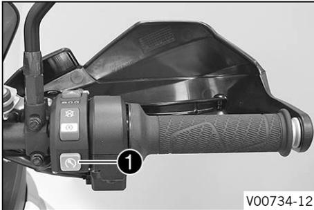
The Race-on tip switch ① is fitted on the right side of the combination switch.
