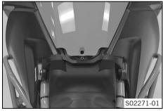
Raise the tank cover at the rear and take it off in a forward direction.
