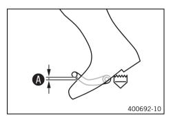
Sit on the vehicle in the riding position and determine distance A between the upper edge of your boot and the shift lever.
