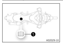
Diagnostics connector is located under the front rider's seat.
