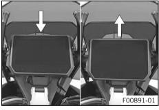
To move the combination instrument to the desired position, press the combination instrument upward or downward.
