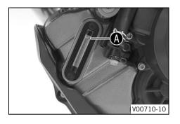
Add engine oil to the upper marking (A) on the engine oil level viewer.
