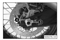
Remove nut 3. Remove chain adjuster 4.
