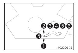
The gear positions can be seen in the figure. The idle position is between the first and second gears.
