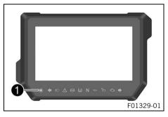
The Race-on indicator lamp 1 can indicate errors by flashing. The flashing occurs for up to five seconds after actuating the Race-on tip switch.
