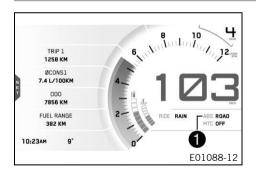
The ABS mode setting is shown in the **1** area of the display. The **ABS** can be configured in the **ABS** menu.
