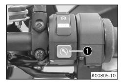
The Race-on tip switch is fitted on the right side of the combination switch
