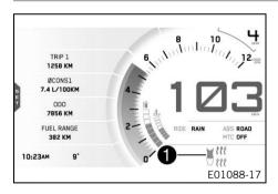
When the seat heating is switched on, the **Heated Seat** symbol appears in the **1** area of the display.
