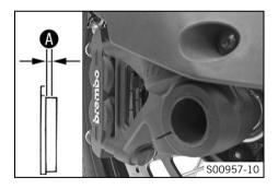
Check all brake linings on both brake calipers to ensure they have minimum thickness **A**.
