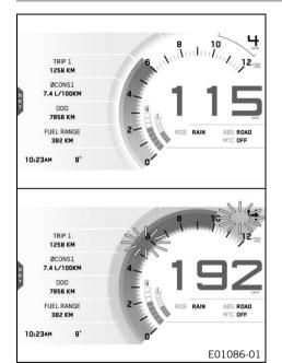
The shift warning light is integrated in the tachometer display. In the **Shift Light** menu, the engine speed for the shift warning light can be set. The shift warning light is always active during the running-in phase (up to 1,000 km / 621 mi). The shift warning light can only be deactivated, and the values for **RPM1** and **RPM2** can only be adjusted after this. The shift warning light lights up red at **RPM1** and flashes red at **RPM2**.
