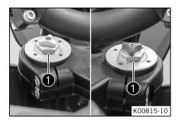
Turn adjusting screws 1 counterclockwise all the way.
