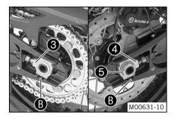
Push the wheel spindle in all the way and mount chain adjuster 4 and nut 5.
