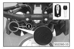
On this vehicle, the ignition/steering lock is replaced by a remote key with transponder (Race-on key () p. 43)).
