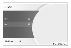
The motorcycle traction control (MTC) lowers the engine torque in case of loss of traction in the rear wheel. Depending on the motorcycle traction control setting, a slight slip on the rear wheel may be desirable. Example: offroad.
