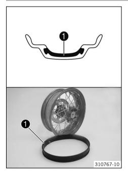
This vehicle makes use of a tubeless tire system in which a tubeless sealing profile **1** is used instead of the conventional tube. The advantage of the tubeless system is that there is no risk of a defective tube. This greatly reduces the risk of a sudden loss in pressure.
