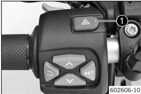
The hazard warning flasher switch ❶ is fitted on the combination switch on the left.
