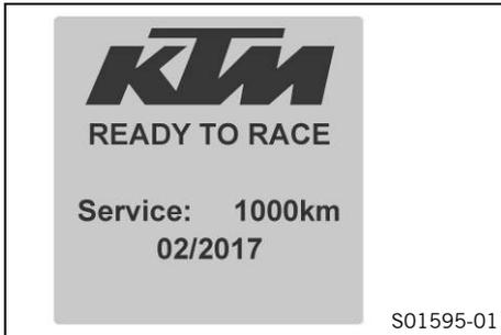
The matrix display is controlled using the menu switch (📖 p. 34). After the ignition is switched on, the display shows when the next service (📖 p. 60) is due.
