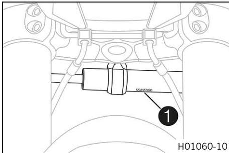
Steering damper item number ① is embossed on the underside of the steering damper.
