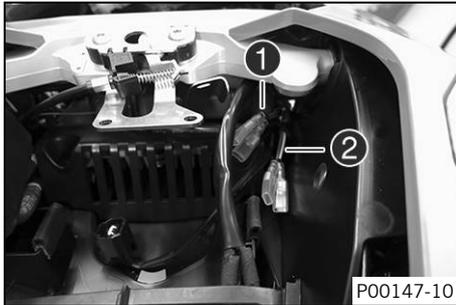
The rear power supplies ACC1 ① and ACC2 ② are located on the right next to the passenger seat lock.
