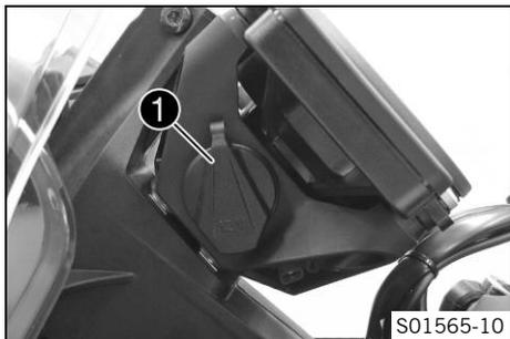
Socket ❶ for electrical accessories is mounted on the left side of the instrument support. It is connected to the permanent positive and is fuse-protected.
