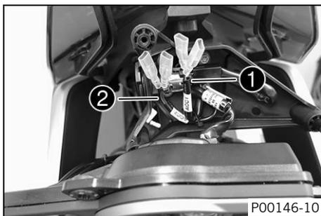
The front power supplies ACC1 **1** and ACC2 **2** are located at the front behind the combination instrument.
