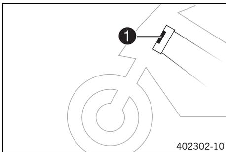
The type label **1** is located on the steering head.
