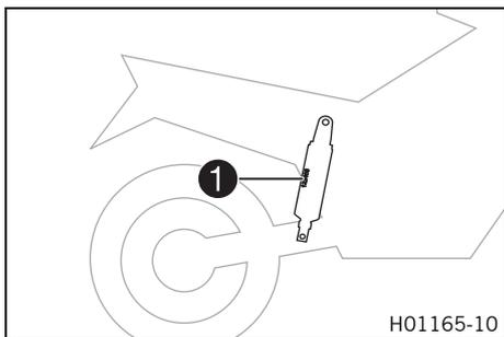
The shock absorber article number **1** is printed on a sticker on the shock absorber case under the spring.
