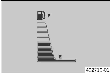
The fuel level display shows the filling level of the fuel tank.
