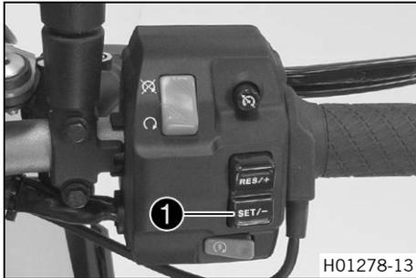
Lower button ① of the cruise control system is fitted on the right side of the combination switch.
