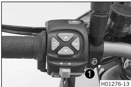
Turn signal switch ① is fitted on the combination switch on the left.
