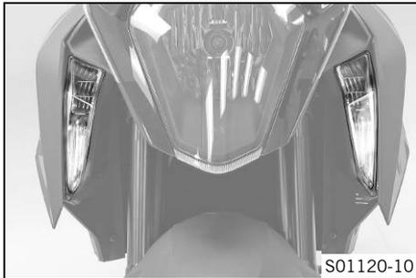
The cornering headlight is located on the left and the right in the tank spoiler.
