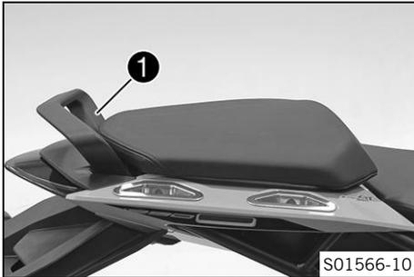
The passenger can hold onto the grab handle **1** during the trip.
