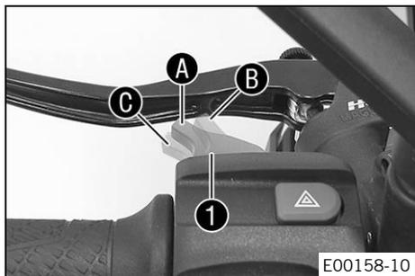
The light switch ❶ is fitted on the combination switch on the left.
