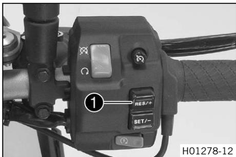
Upper button ❶ of the cruise control system is fitted on the right side of the combination switch.
