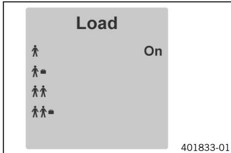
Tunings for different vehicle loading states can be selected in the **"Load"** menu. A selection can be made between one-person operation, one-person operation with luggage, two-person operation, and two-person operation with luggage.
