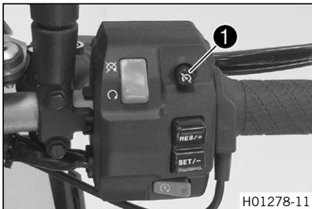
Switch ❶ for the cruise control system is fitted on the right of the combination switch.
