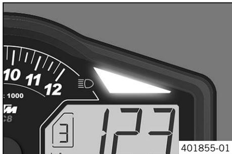
The shift warning light flashes or lights up when the transmission should be shifted.
