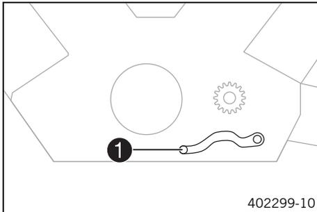
The shift lever **1** is fitted on the left side of the engine.
