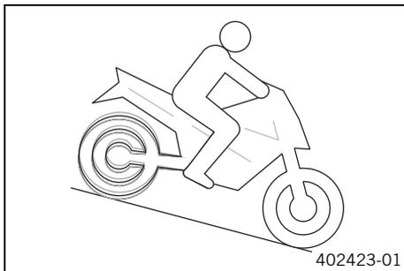
The **MSR** is an optional auxiliary function of the engine control. If the engine braking effect is too great, the **MSR** prevents the rear wheel from locking or sliding away on a sloping position. To avoid slip of the rear wheel, the **MSR** only opens the throttle valve as far as absolutely necessary. The **MSR** is applied on surfaces, where the friction is too low to open the anti-hopping clutch. To further increase ride safety, the **MSR** is slope dependent.
