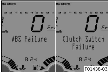
**ABS Failure** appears on the display if the ABS is no longer active.
