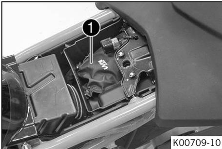
The tool set ① is in the storage compartment under the seat.
