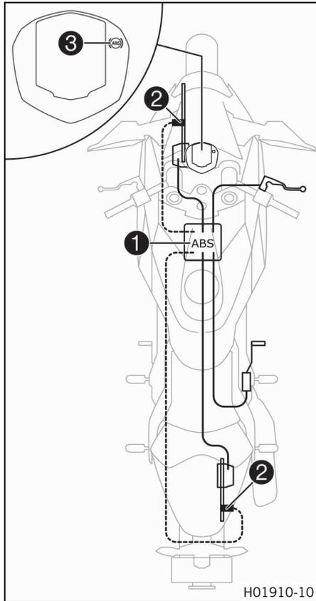
The ABS unit **1**, which consists of a hydraulic unit, ABS control unit, and return pump, is installed under the seat. One wheel speed sensor **2** is located in each case on the front and the rear wheel.
