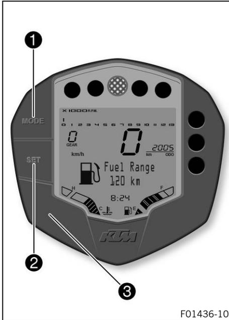
Press the **MODE** button **1** to change display modes. Possible display modes are **TRIP F** (after reaching the fuel reserve level), **Error**, total distance traveled (**ODO**), distance 1 (**TRIP 1**) and distance 2 (**TRIP 2**).
