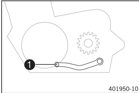
Shift lever ① is mounted on the left side of the engine.
