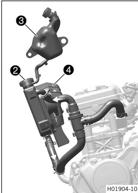
The coolant is cooled by the air stream and a radiator fan **4**, which is activated at high temperature. The lower the speed, the less the cooling effect. Dirty cooling fins also reduce the cooling effect.
