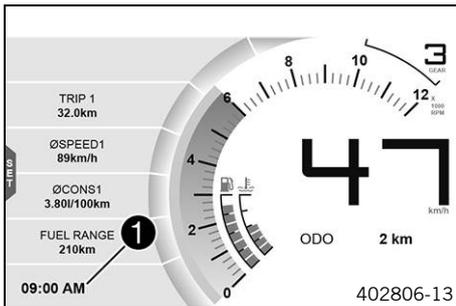
The time is shown in area ❶ of the display. The time is displayed in 24 hour format in all languages except for EN-US. The time is displayed in 12 hour format if the language is set to EN-US. The time can be configured in the **Clock/Date** menu.
