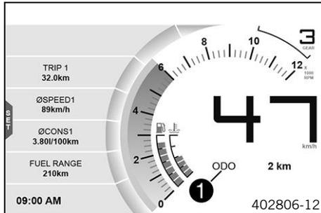
The total distance covered **ODO** is shown in area **1** of the display.
