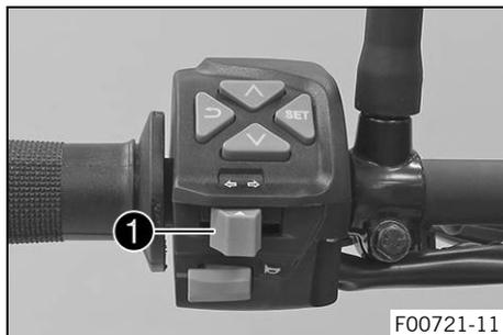
Turn signal switch **1** is fitted on the left side of the handlebar.
