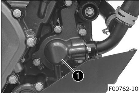
Water pump ① in the engine ensures forced circulation of the coolant.
