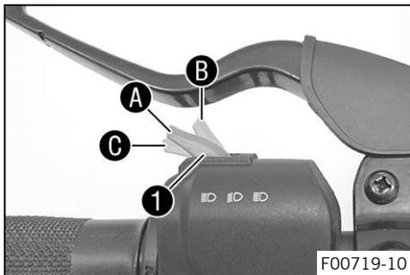
Light switch ① is fitted on the left side of the handlebar.
