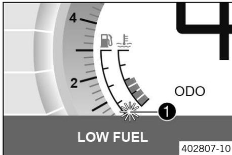
The fuel tank contents are shown in area **1** of the display. The fuel level indicator consists of bars. The more bars are lit, the more fuel is in the fuel tank.
