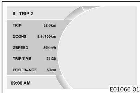
When the menu is closed, the **Quick Selector 2** menu is opened by pressing the **DOWN** button. Press the **BACK** button to close **Quick Selector 2**.
