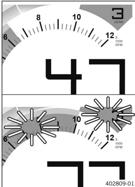
The shift warning light is integrated in the tachometer display. In the **Shift Light** menu, the engine speed for the shift warning light can be set. The shift warning light is always active during the running-in phase (up to 1,000 km / 621 mi). The shift warning light can only be deactivated, and the values for **RPM1** and **RPM2** can only be adjusted after this. The shift warning light lights up red at **RPM1** and flashes red at **RPM2**.
