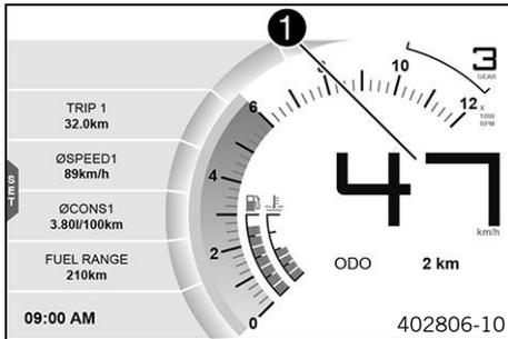
Speed ① is shown in kilometers per hour **km/h** or in miles per hour **mph**.
