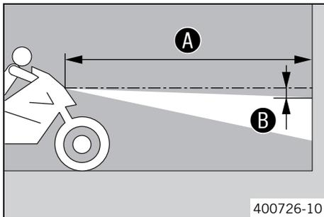
– Position the vehicle upright on a horizontal surface in front of a light wall and make a marking at the height of the center of the low beam headlight.
