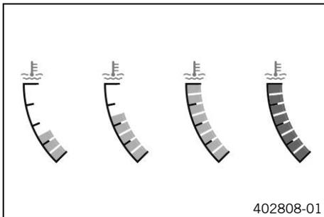
The coolant temperature indicator consists of bars. The more bars that light up, the hotter the coolant.
