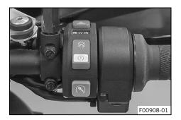
Turn the emergency OFF switch/electric starter button to the lower position (3).
