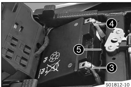
3.6 Installing the battery
