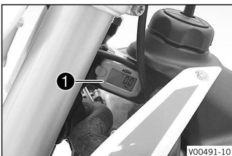
The service hour counter ❶ is fitted on the left side of the frame. It shows the total number of service hours of the engine. The service hour counter begins counting when the engine is started and stops when the engine is switched off.
