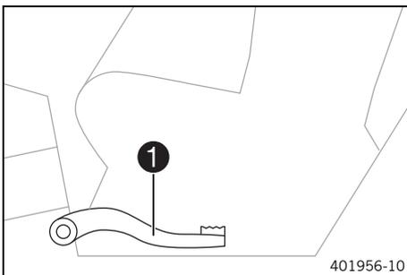
Foot brake lever ❶ is located in front of the right footrest. The rear brake is engaged with the foot brake lever.
