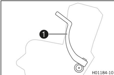
Kick starter ❶ is fitted on the right side of the engine. The kick starter can be swiveled.
