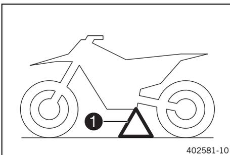
The fixture for plug-in stand ❶ is located on the frame on the left side of the vehicle. The plug-in stand is used to park the motorcycle.
