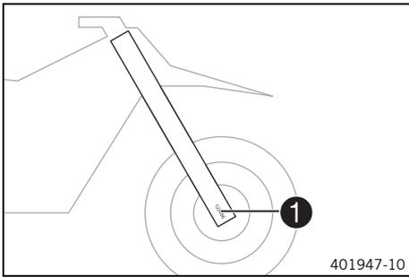
The fork part number **1** is stamped on the outside of the axle clamp.
