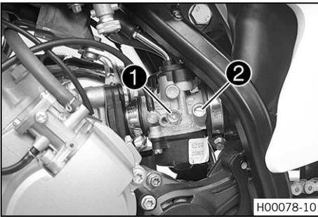
The idle setting of the carburetor has a big influence on the starting behavior, stable idling, and the response to throttle opening. This means that an engine with a correctly set idle speed is easier to start than if the idle speed is set wrongly.
