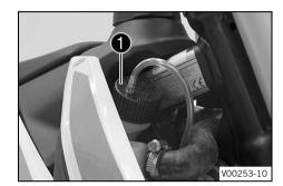
Turn the oil tank cap 1 counterclockwise and pull it up.
