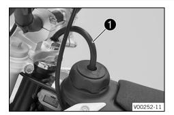
Mount the filler cap and turn it clockwise until the fuel tank is firmly closed.
