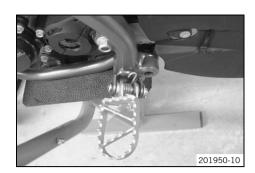
Mount the footrests with the springs and pins. Secure the pins using the washers and cotter pins.
