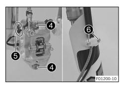
Position the brake caliper. Mount and tighten screws 4 with the spacers.
