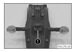
Position the license plate lamp on the license plate holder extension, and mount and tighten screw 1.
