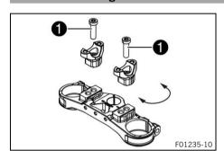
Remove screws 1. Take off the handlebar supports.
