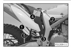
Push splash protector 1 to the side and position the shock absorber. Mount and tighten screw 2.
