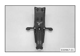
Position the turn signal on both sides on the license plate holder, mount nuts with washers and tighten.
