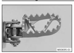
Mount the left footrest and the right footrest with the springs and pins. Secure the pins using the washers and cotter pins.
