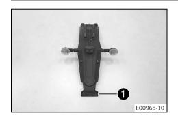
Mount reflector on the license plate holder with the spring washer.
