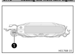
Position turn signal indicator lamp 1 in the combination instrument rack.
