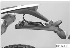
Route turn signal cable to the rear through the license plate holder extension.
