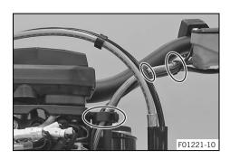
Route the cables without tension and secure with cable ties and cable holders.
