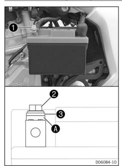
Connect negative cable of the 12 V battery.
