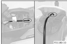
Route the turn signal cable harness through the frame from the front to the rear paying attention to the plugs as you do so.
