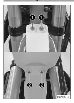
Position front fender. Mount and tighten screws ①.
