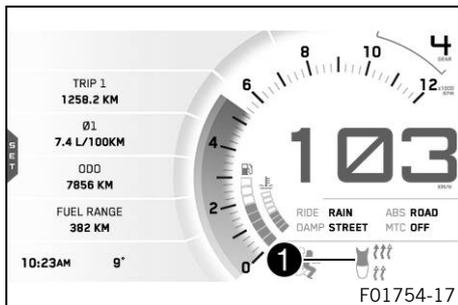
When the seat heating is switched on, the **Heated Seat** symbol appears in area ❶ of the display.
