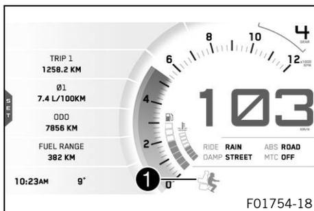
The payload setting is shown in area ❶ of the display.
