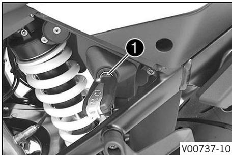
Seat lock ① is located on the left side of the vehicle under the seat.
