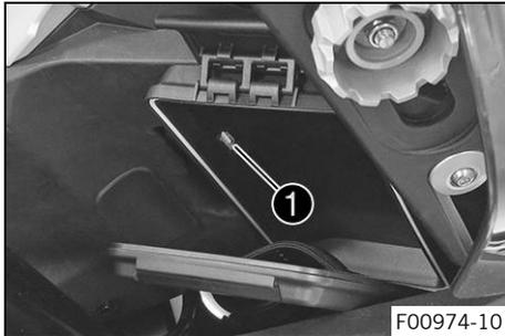
A USB socket **1** is located in the storage compartment for supplying power to external devices. The USB socket is activated when the ignition is switched on.
