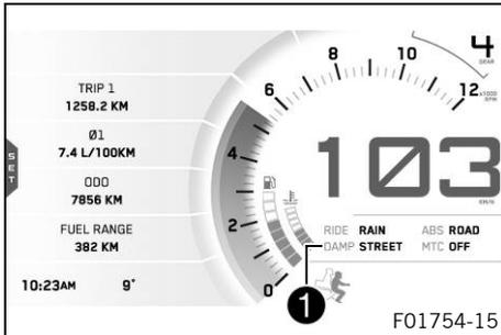
The **Damping** mode setting is shown in the ❶ area of the display. The damping can be configured in the **Damping** menu.
