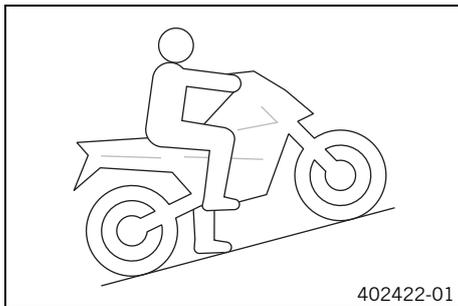
The **HHC** is an optional auxiliary function of the brake system. The **HHC** prevents accidental rolling back of the motorcycle on hills.
