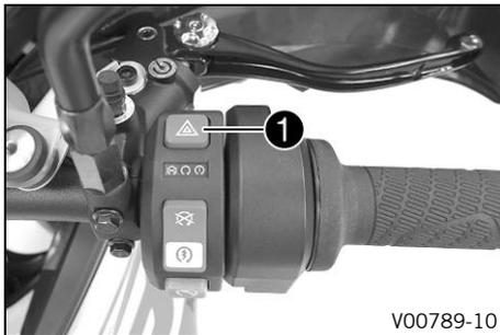
The hazard warning flasher switch ❶ is fitted on the right side of the combination switch. The hazard warning flasher is used to indicate emergency situations.
