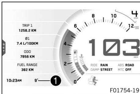
The ambient air temperature is displayed in the ❶ area. The unit of ambient air temperature can be configured in the **Temperature** menu. The ambient air temperature is displayed in °C or °F.
