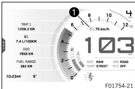
The operating state and active cruise control are shown in the ❶ area of the display.
