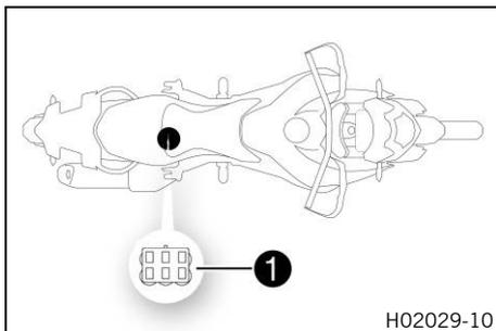
Diagnostics connector ① is located under the front rider's seat.
