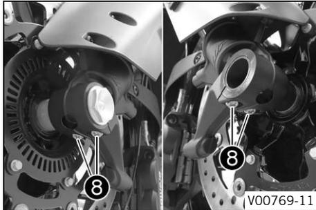
– Operate the front brake and compress the fork a few times firmly.
