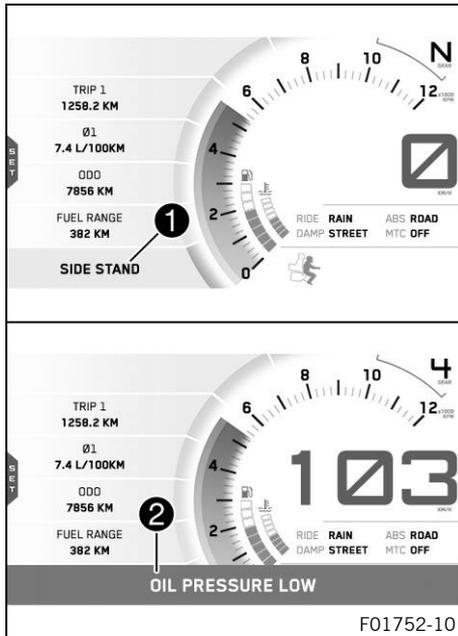
Warnings appear on the bottom edge of the display; these are marked yellow or red depending on their relevance. Yellow warnings ① indicate errors or information which require prompt intervention or an adjustment to the riding style. Red warnings ② indicate errors or information which require immediate intervention.
