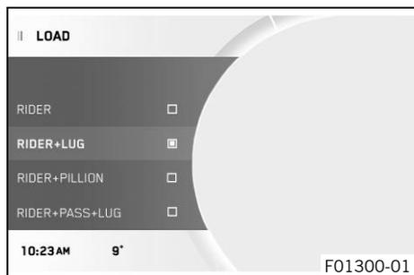
The settings for different payloads can be selected in the **Load** menu. A selection can be made between one-person operation, one-person operation with luggage, two-person operation, and two-person operation with luggage.
