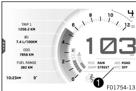
The **Ride Mode** setting is shown in area **1** of the display. The drive mode can be configured in the **Ride Mode** menu.
