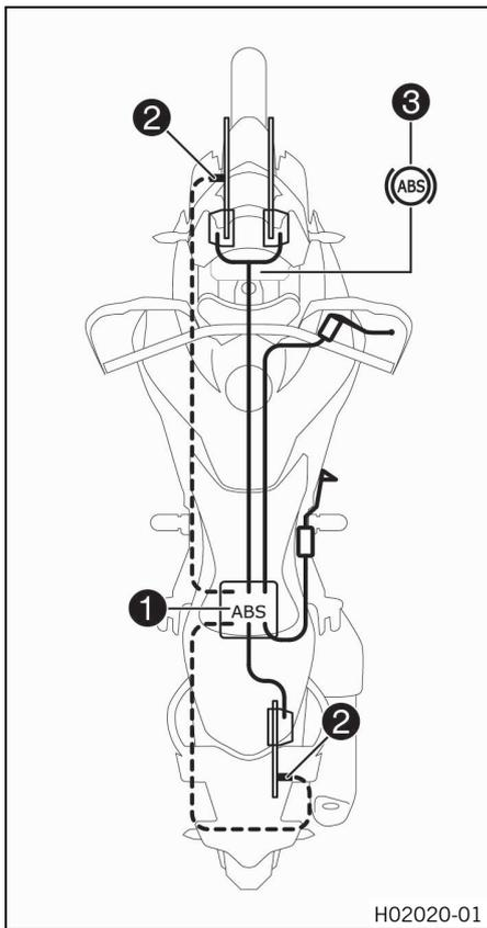
The ABS module **1**, consisting of a hydraulic unit, brake electronics control unit, and a return pump, is located under the seat. One wheel speed sensor **2** is located in each case on the front and the rear wheel.
