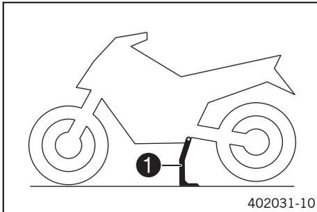
In addition to the side stand, the vehicle is equipped with a center stand **1**.
