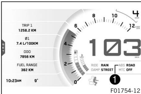
The ABS mode setting is shown in the **1** area of the display.
