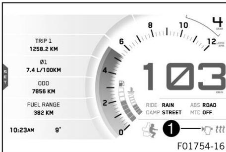
When the heated grip is switched on, the **Heated Grips** symbol appears in the ❶ area of the display. The heated grip can be configured in the **Heated Grips** menu.
