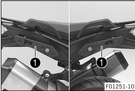
Case holders **1** are located on each side of the passenger seat. A case system (optional) can be attached on the case holders. Use case systems approved and/or recommended by KTM. Observe the specifications in the enclosed **KTM PowerParts** fitting instructions.
