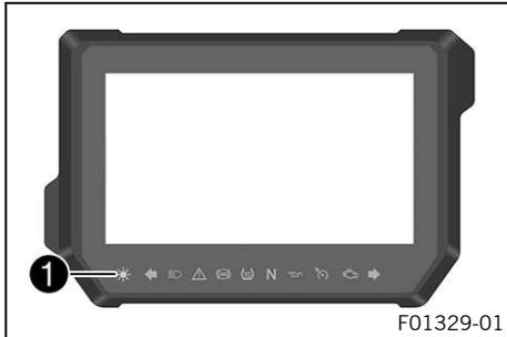
The Race-on indicator lamp **1** can indicate errors by flashing. These are indicated up to five seconds after the Race-on tip switch is actuated.
