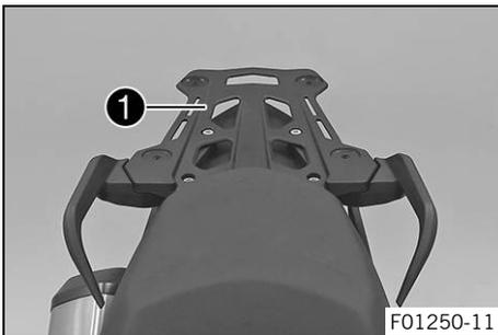
The luggage rack plate **1** is located behind the seat. The base plate of a luggage system (optional) can be attached to the luggage rack plate. The luggage rack plate may not be loaded with more than the specified weight.
