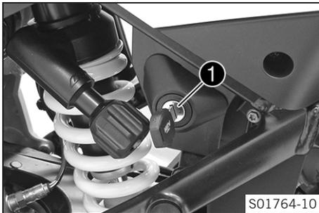
The seat lock **1** is located on the left side of the vehicle. It can be unlocked using the ignition key.
