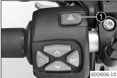
The hazard warning flasher switch ① is fitted on the combination switch on the left.
