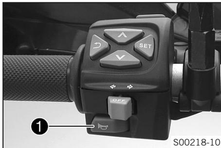
The horn button **1** is fitted on the combination switch on the left.
