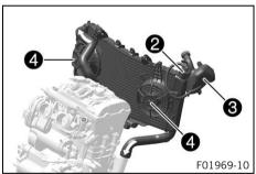
The coolant is cooled by the air stream and two radiator fans **4**, which are activated at high temperature.
