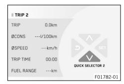
When the menu is closed, the **Quick Selector 2** display is opened by pressing the **DOWN** button.
