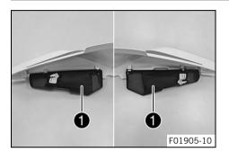
The left or right storage compartment contains the on-board tool set  $\ensuremath{\text{\textbf{0}}}$ .
