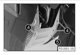
Remove screws 4 and engine guard 5.
