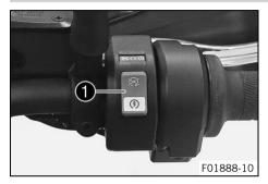
The emergency OFF switch/electric starter button **1** is located on the right side of the combination switch.
