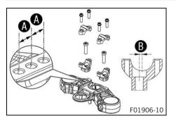
On the upper triple clamp, there are three holes at a distance of  $\bf A$  to each other.
