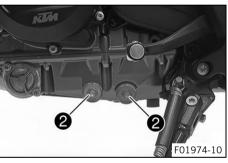
Mount the oil drain plugs 2 with magnets and new seal rings, and tighten.
