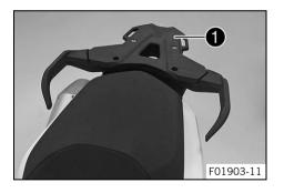
The luggage rack plate 1 is located behind the passenger seat. The base plate of a luggage system can be mounted on the luggage rack plate (optional).
