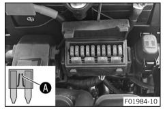
Remove the faulty fuse.
