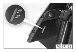
Check the coolant level in the compensating tank  $oldsymbol{1}$ .
