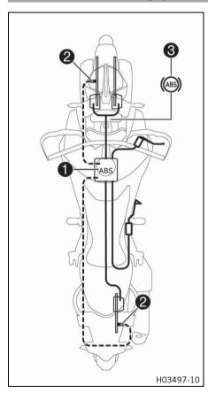
The ABS module ①, which consists of a hydraulic unit, ABS control unit, and return pump, is installed under the fuel tank. One wheel speed sensor ② is located in each case on the front and the rear wheel.
