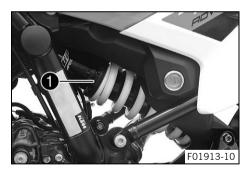
Adjust the spring preload by turning adjusting ring using the hook wrench from the tool set.
