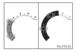
The shift warning light is integrated in the tachometer display. In the **Shift Light** submenu, the engine speed for the shift warning light can be set. The shift warning light is always active during the running-in phase (up to 1,000 km / 621 mi). The shift warning light can only be deactivated, and the values for **Lights up** and **Flashes** can only be adjusted after this. In **Lights up** the shift warning light flashes and in **Flashes** it flashes and the color changes.
