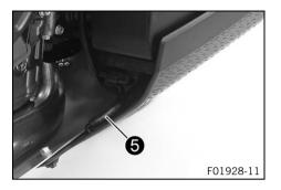
Attach tube 6 to the angle piece.
