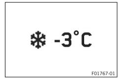
The ice warning \* appears on the display when the ambient temperature drops below the specified value.
