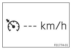
When cruise control is activated, the operating mode is shown on the combination instrument display.
