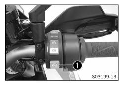
The <u>Race-on tip switch</u> is fitted on the right side of the combination switch.
