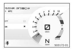
The motorcycle traction control ( $\underline{MTC}$ ) lowers the engine torque in case of loss of traction in the rear wheel.
