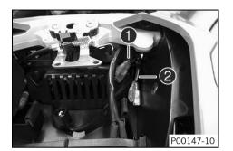
The rear power supplies ACC1 1 and ACC2 2 are located on the right next to the passenger seat lock.
