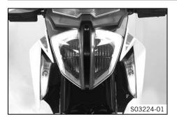
The cornering light is located on the left and the right in the fuel tank spoiler.
