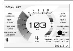
The **Ride Mode** setting is shown in area **1** of the display. The drive mode can be configured in the **Ride Mode** menu.
