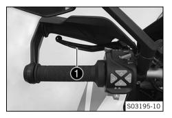
Clutch lever **1** is fitted on the handlebar on the left. The clutch is activated hydraulically and adjusts itself automatically.
