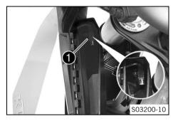
A USB socket **1** for supplying power to external devices is located in the left storage compartment.
