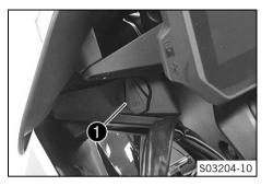
Socket **1** for electrical accessories is mounted on the left side of the instrument support.
