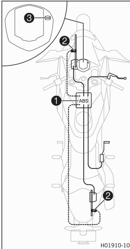
The ABS module **1**, consisting of a hydraulic unit, an ABS control unit, and a return pump, is located under the seat. One wheel speed sensor **2** is located in each case on the front and the rear wheel.
