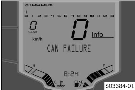
If an error has occurred in the CAN bus, various warnings appear on the display:
