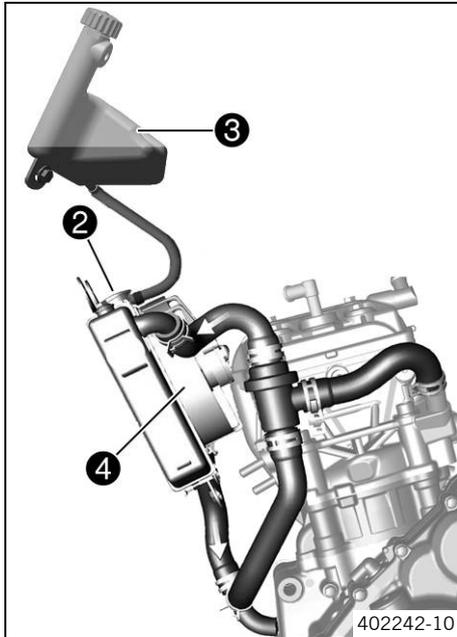
The coolant is cooled by the air stream and a radiator fan **4**, which is controlled by a thermostatic switch. The lower the speed, the less the cooling effect. Dirty cooling fins also reduce the cooling effect.
