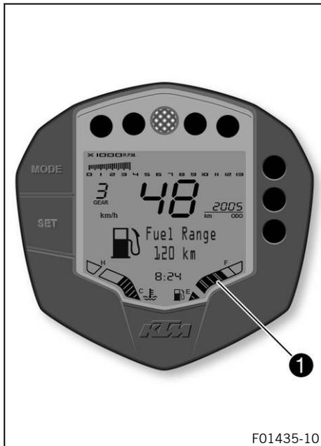
The fuel tank contents are shown in area ❶ of the display. The fuel level indicator consists of bars. The more bars are lit, the more fuel is in the fuel tank.
