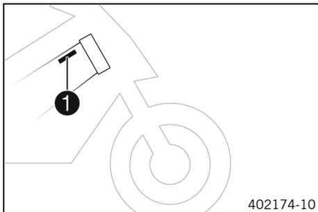
The vehicle identification number **1** is stamped on the right of the frame behind the steering head.
