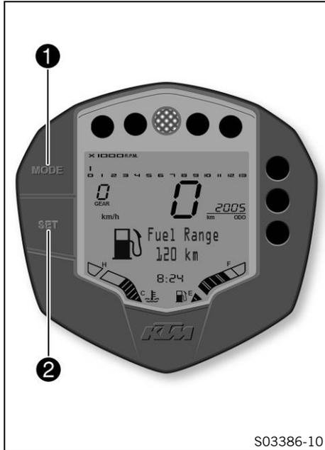
Press the **MODE** button **1** to change display modes. Possible display modes are **TRIP F** (after reaching the fuel reserve level), **Info**, total distance traveled (**ODO**), distance 1 (**TRIP 1**) and distance 2 (**TRIP 2**).
