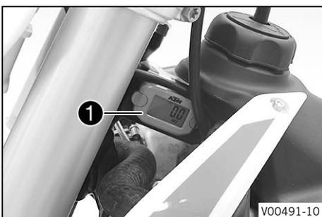
The service hour counter ❶ is fitted on the left side of the frame. It shows the total number of service hours of the engine.
