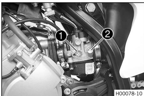
The idle setting of the carburetor has a big influence on the starting behavior, stable idle speed, and the response to throttle opening. This means that an engine with a correctly set idle speed will be easier to start than one with an incorrectly set idle speed.
