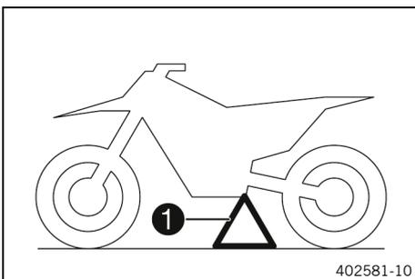
The fixture for plug-in stand ❶ is located on the frame on the left side of the vehicle.
