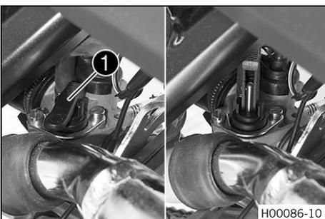
The choke lever **1** is fitted on the right of the carburetor. Activating the choke function frees a drill hole in the carburetor through which the engine can draw extra fuel. This results in a richer fuel-air mixture, which is needed for a cold start.
