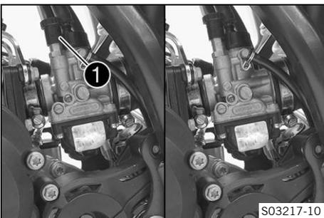
Choke **1** is fitted on the left side of the carburetor. Activating the choke function frees a drill hole in the carburetor through which the engine can draw extra fuel. This results in a richer fuel-air mixture, which is needed for a cold start.
