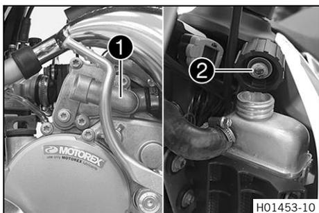
The water pump ① in the engine forces the coolant to flow. The pressure resulting from the warming of the cooling system is regulated by a valve in the radiator cap ②. This ensures that operating the vehicle at the specified coolant temperature will not result in a risk of malfunctions.
