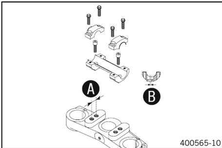
On the upper triple clamp, there are 2 holes at a distance of **A** to each other.
