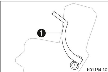
Kick starter lever ❶ is fitted on the right side of the engine. The kick starter lever can be swiveled.
