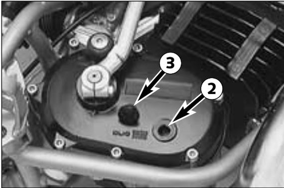
Lay the motorcycle on its side and add 0.25 l gear oil SAE 30 (ex. Shell Advance VSX 4). Mount the plug ❸ and check the engine for leaks.
