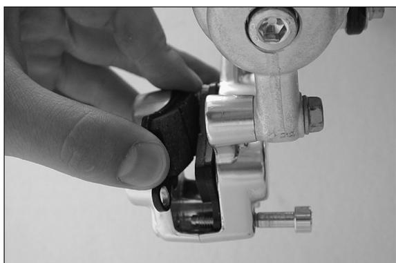
Mount the right brake shoe and fix with screw. Mount the left brake shoe and tighten the screw to 10 Nm. Mount the lock washer. Align brake shoes, mount front wheel (see chapter: Mounting the front wheel).
