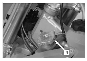
A mixture of 50% antifreeze liquid and 50% water is used as coolant. However, the antifreeze protection must be at least -25° C (-13° F). This mixture offers antifreeze protection but also good corrosion protection and should therefore not be replaced by pure water.
