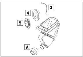
Thoroughly wash the foam filter in special cleaning fluid and allow to dry well. Only press out the filter, do not wring out under any circumstances. Oil the dry foam filter with a high grade filter oil. Also clean the air filter box. Check carburetor collar [A] for damage and that it is fitted correctly.
