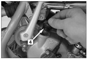
Remove the filler plug [4] and add 0.30 I gear oil 20W30 (e.g. Motorex Top Speed 4T 15W50). Mount the filler plug and check the engine for leaks.
