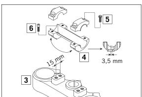
For this purpose, remove screws [5] of the handlebar clamps and screws [6] of the handlebar support. Position handlebar support, and tighten screws [6] to 40 Nm. Mount handlebar and handlebar clamps, and tighten screws [5] to 20 Nm. The gap between the handlebar support and handlebar clamps should be the same size in the front and in the rear.
