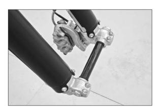
Loosen the clamping screws on the fork leg axle passages and remove the wheel spindle.
