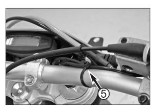
Attach the cable to the handlebar with a cable clip 6.
