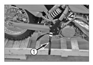
Carefully relieve the rear tensioning strap and remove while holding the motorcycle handlebar.
