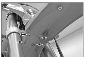
Screw on the 4 fender fixing screws (M6x20, included in the kit "Umrüstung") and tighten.
