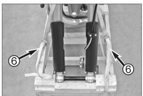
Carefully loosen the front tensioning straps 6 and remove.
