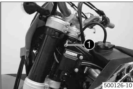
Steering lock ❶ is fitted on the left side of the steering head.
