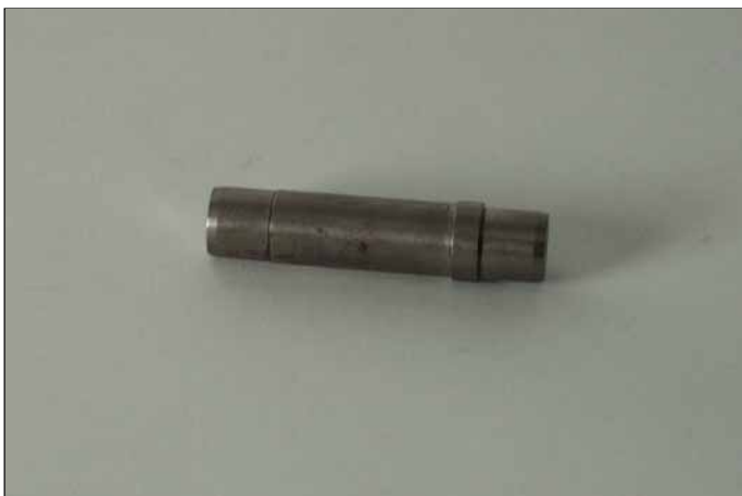
T14.022. Dis- / assembling tool DU-bush d12.
