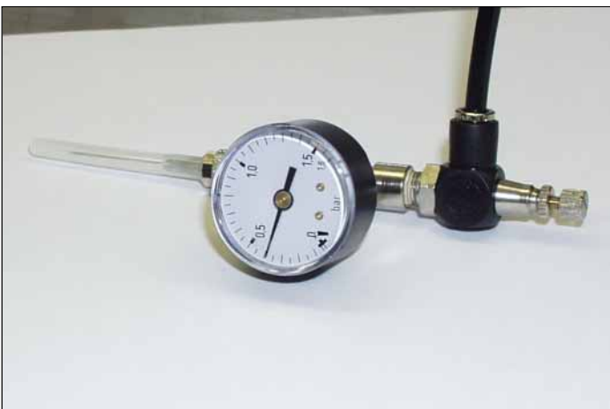
T14.019. Charging device tool.
