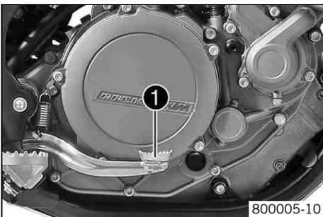
Foot brake pedal ❶ is located in front of the right footrest. The foot brake pedal is used to activate the rear brake.
