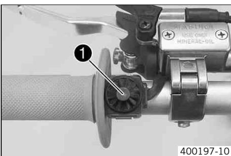
Short circuit button ❶ is fitted on the left side of the handlebar.
