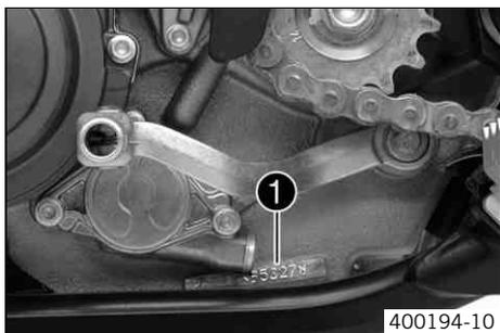
The engine number ❶ is stamped on the left side of the engine under the engine sprocket.
