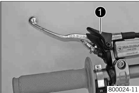
The hot start lever ❶ is fitted on the left side of the handlebar. If you pull the hot start lever to the handlebar during the start procedure, a bore is opened in the carburetor through which the engine can draw in extra air. This gives a leaner fuel-air mixture, which is needed for a hot start.
