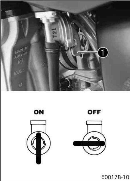
The fuel tap is on the left side of the fuel tank. Using tap handle ❶ on the fuel tap, you can open or close the supply of fuel to the carburetor.
