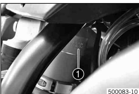
The shock absorber part number ❶ is stamped on the top of the shock absorber above the adjusting ring on the engine side.
