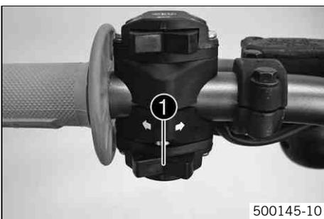
Flasher switch ❶ is fitted on the left side of the handlebar.
