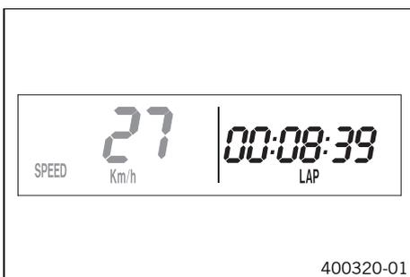
– Press the button
