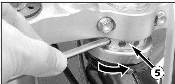
To adjust, loosen the clamping screws ⑤ on the fork stabilizers. Insert a pin (6 mm) in the adjusting nut ⑥ and turn the fork tube 180° in a counter-clockwise direction (not clockwise or you will change the positioning of the steering head bearings). The groove A must match the slot on the upper triple clamp. Tighten the clamping screws to 20 Nm.
